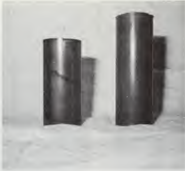
FIGURE 13. FRACTURED BIAXIAL SPECIMEN CASTINGS.
